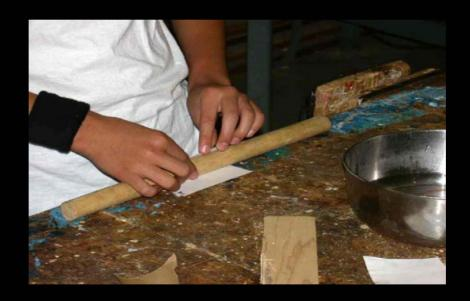
Reinforce tube with paper tape attached parallel to edge of dowel.
